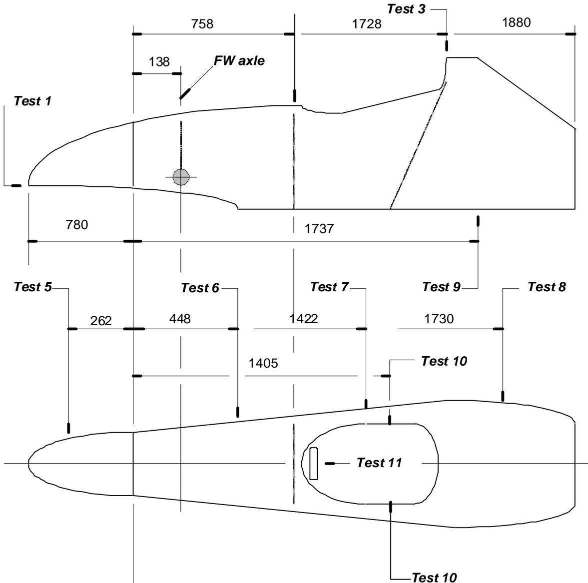
**Test 1 : A frontal impact test against a solid barrier at 12 metres/sec with a total mass of 650kg**
