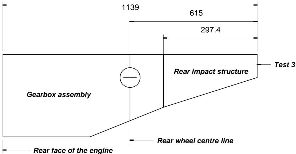
**Test 2c: An impact test against a solid barrier at 10 metres/sec with a total mass of 560kg**
