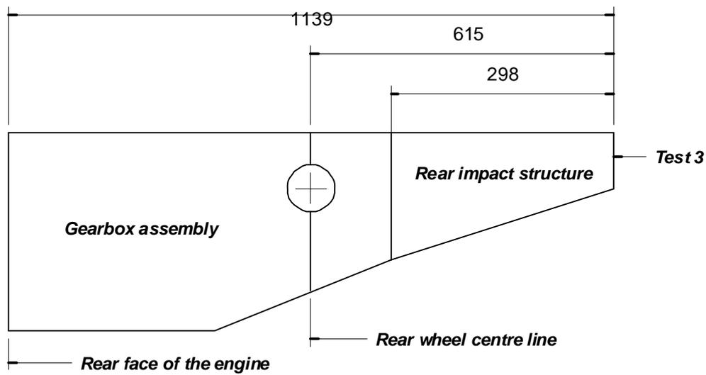
**Test 3 : A 83.55kN or 66.84kN load applied at a compound angle to the top of the main roll structure**
