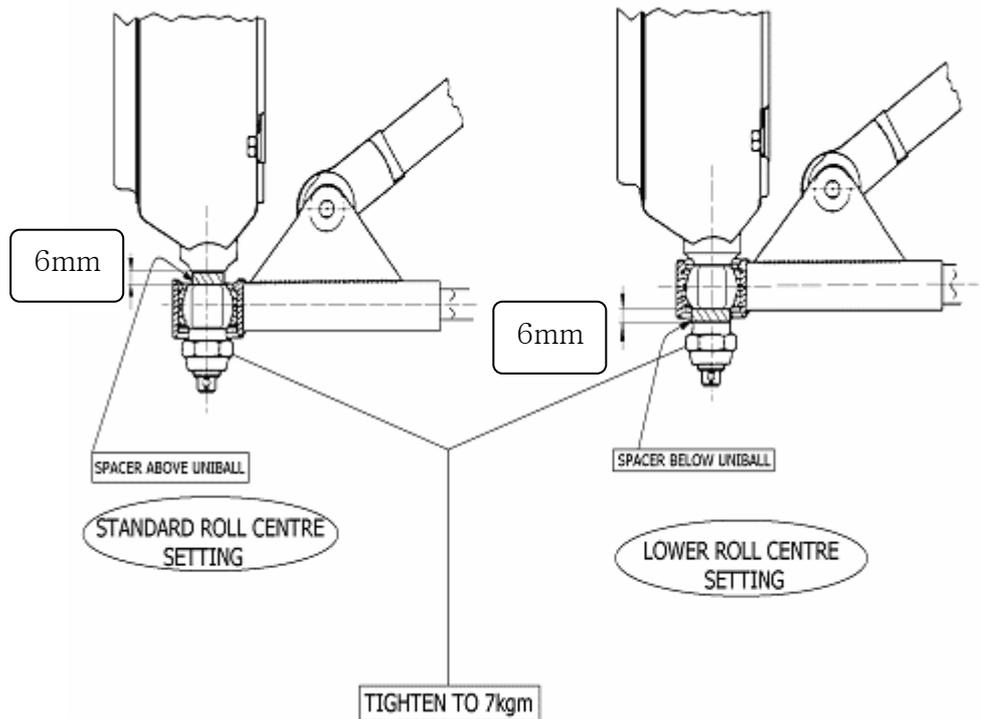
The drawing shows the roll centre setting on WMP. The procedure and effect are identical on UMP suspension.
