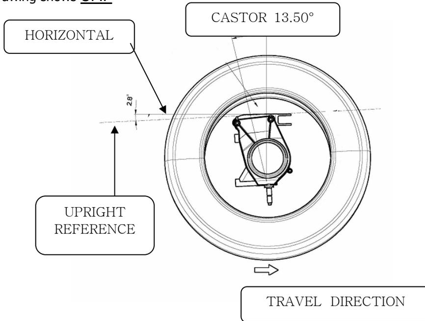
**When the car has a pitch angle**, that is with different front and rear ride height.
