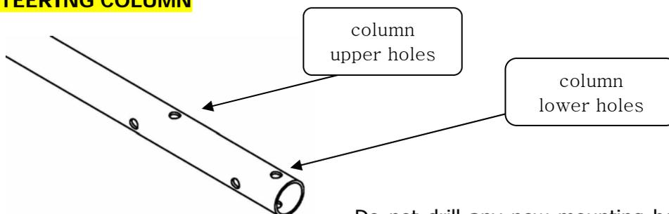
Do not drill any new mounting holes further up the column than the upper holes standard made by Dallara.
